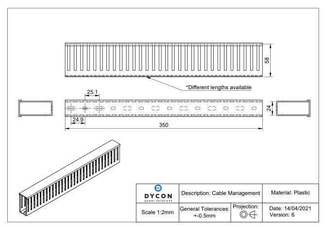
Designed to group and tidy up various cables inside a Dycon housing. The slots enable individual cables to be fed out near to the point at which they are to be terminated or connected, reducing the number of cables sitting near any electronic units. The top is easily opened making additions and alterations quick and simple without disturbing
